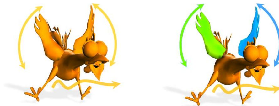
Fig. 13 Chicken dynamic mesh movement simplification. Three important movements for each vertex of chicken mesh on the left. On the right clustered chicken mesh with only one important movement for torso and each wing.
