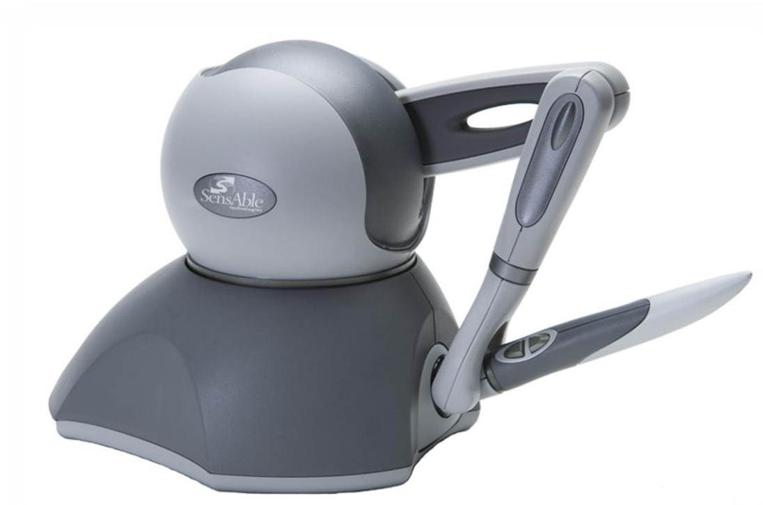
Obrázek 1: Phantom Omni Haptic Device [3]
