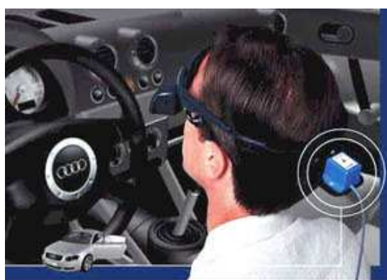
3D-BIRD mounted on Sony LDI-100 HMD. Audi TT Coupe virtual interior and exterior environment courtesy Eon Reality, Sweden.
