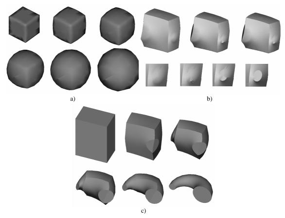
**Figure 4.8:** A morphing animation rendered so that: a) sharp edges were not considered, b) normals recomputed in each animation frame, c) normals computed using the face mapping approach.
