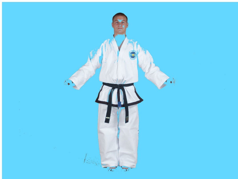
Figure A.3: RGB difference matte. Foreground object is full of holes. However if we would lower the difference threshold, shadows from background will come up
