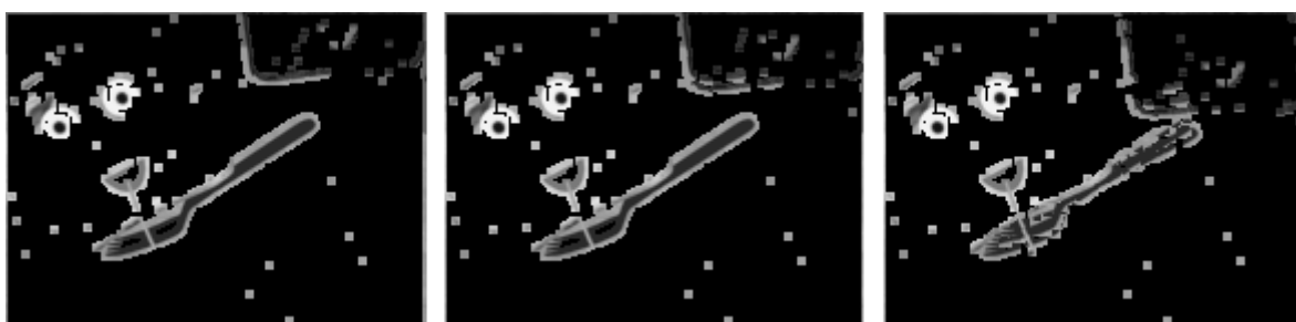
Obr. 7.7: Test odhadu pohybu algoritmem block matching
