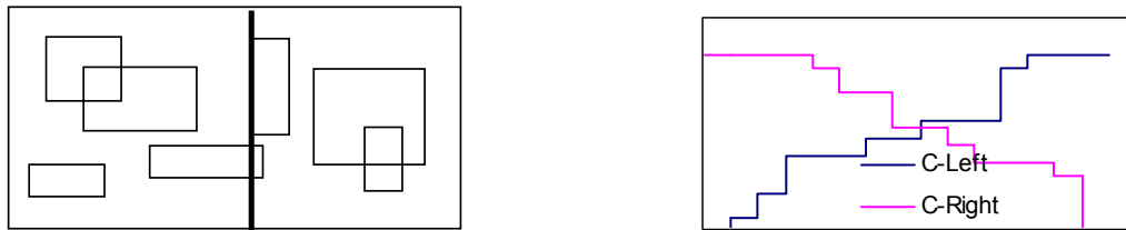
a) bounding boxes in the region and the optimal position of the cut b) estimated costs of the rendering of the left and the right part
