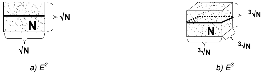
Figure 8.3: The cut of an object containing N uniformly distributed points has approximately square root of N points in its vicinity.
