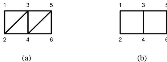
**Figure 7.1:** An example of sequential triangle strip (a) and a sequential quad strip (b).
