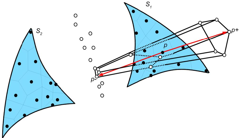
Fig. 4.4: The surface with two parts  $S_1$  and  $S_2$  with the Voronoi cell around the point  $p$  and the medial axis created by other Voronoi vertices (white points). The Voronoi vertices  $p_+$  and  $p_-$  are positive and negative poles of the Voronoi cell.
