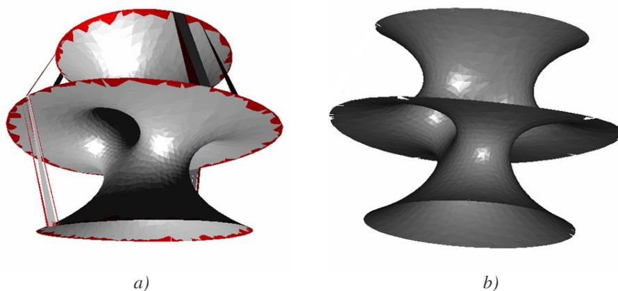
Fig. 9.15: a) The hypersheet model reconstructed by COCONE, the boundary is correctly detected but some incorrect triangles appear, b) our reconstruction, almost all boundary triangles were removed but some of surface triangles, too.
