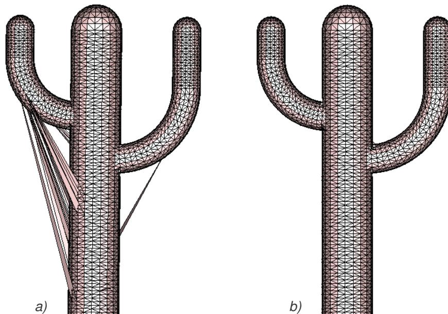
Fig. 5.1: a) An example of the reconstruction without using the numerically stable Delaunay tetrahedronization, b) the reconstruction with numerically stable Delaunay tetrahedronization.
