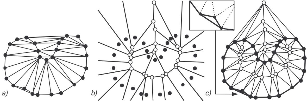
Fig. 4.2: An example of the two-pass curve reconstruction, a) the input point cloud with the Delaunay triangulation, b) the Voronoi diagram with highlighted Voronoi vertices. When we unify the points and Voronoi vertices and triangulate the set, we get the triangulation c) where curve edges (highlighted) incident only with the original points, the box above shows the detail of the problematic area.
