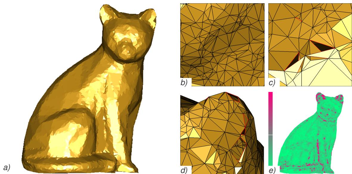
Fig. 5.5: a) An example of a nonuniformly scanned object, b) a detail of the reconstructed triangle mesh, c) the detail of the place with bad triangle configuration, d) the region with a sharp edge and with holes due to a local undersampling (cat's ears), e) the  $\epsilon$ -sampling, darker regions have worse  $\epsilon$ -sampling.
