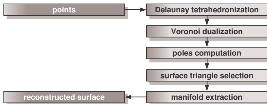
Fig. 6.1: The scheme of the original CRUST algorithm.
