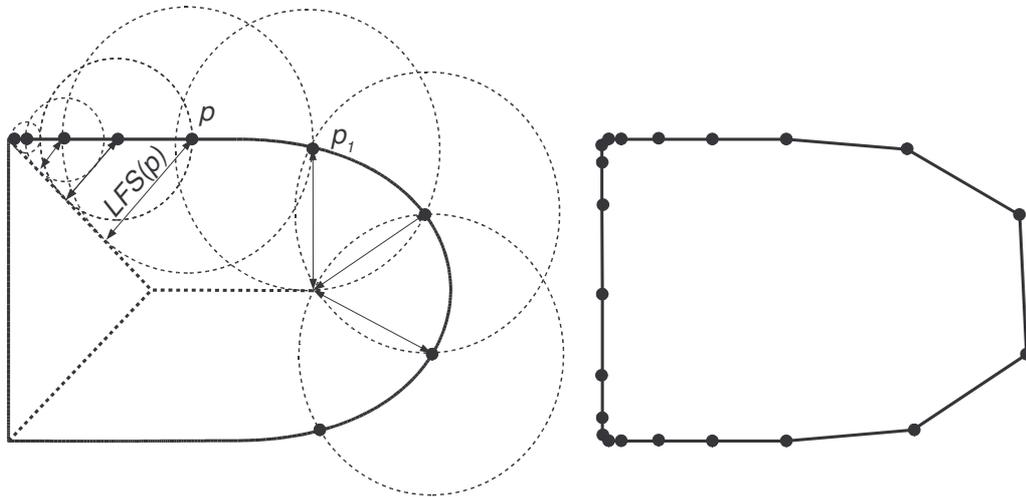
Fig. 1.4: The object and sampling with the local feature size criterion (only a part of the surface sampled is shown for better readability). The circles show the distance to the medial axis and where the closest point should lie. The arrows show the  $LFS$  of the current point. In the right part of the figure the reconstruction is presented, the parts with sharp corners are well reconstructed.
