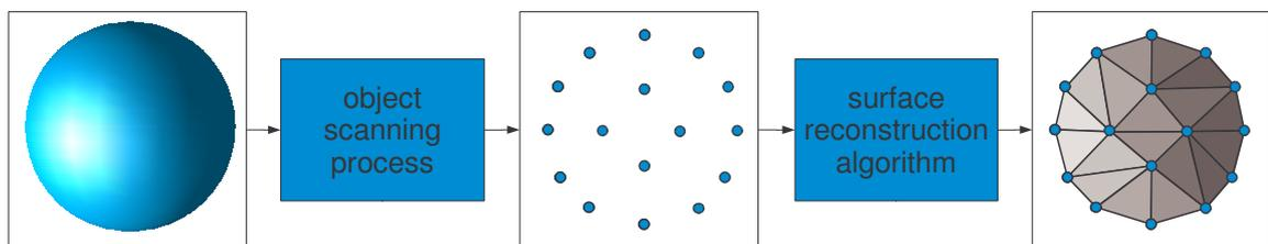
Fig. 1.2: 3D model acquisition pipeline. Some object (the sphere in this example) is scanned and the sampled data is used for the computer model reconstruction.
