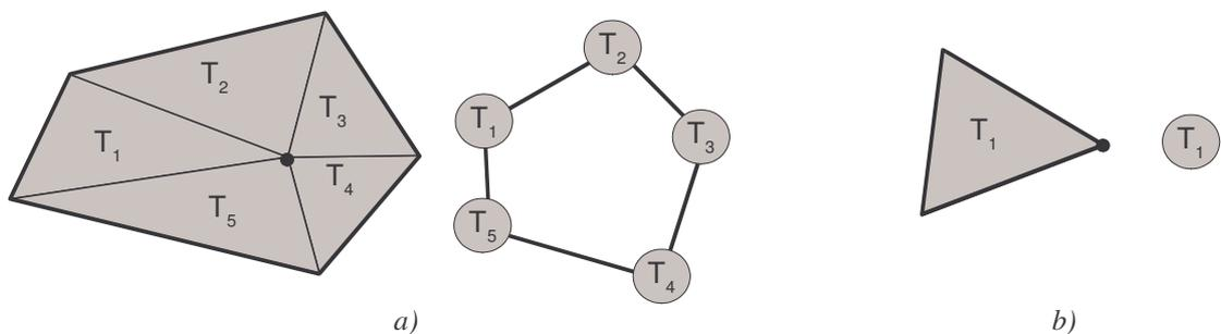
Fig. 9.3: a) Full fan and one graph cycle corresponding to the fan, b) one triangle with its graph.
