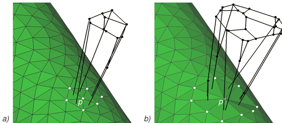
Fig. 4.6: The visualization of the Voronoi cell of the point  $p$ , a) the original dataset, white points will be removed, b) the change of the Voronoi cell shape after removing the points, white points are the vertices of the triangles coincident with the point  $p$ .
