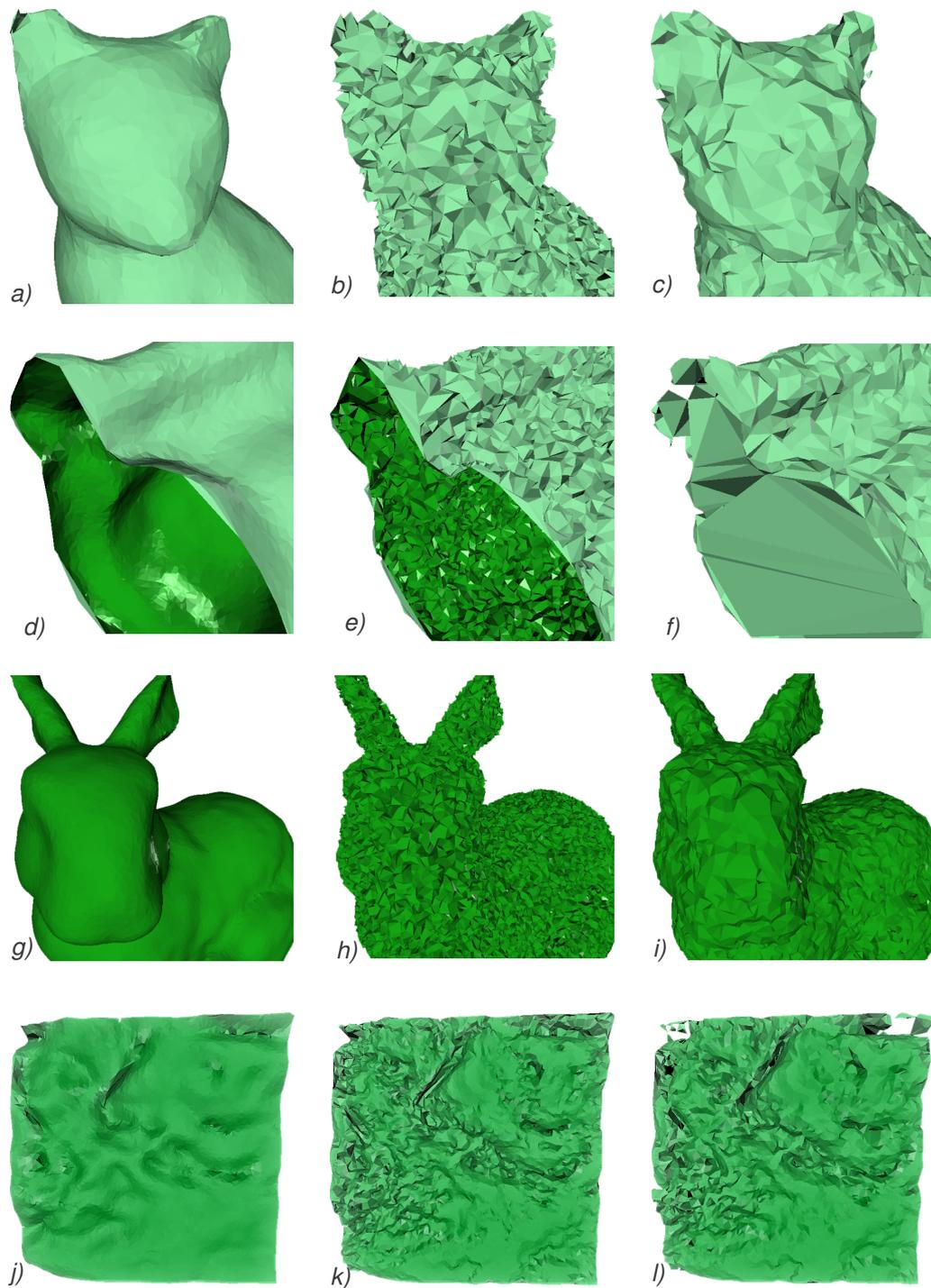
Fig. 7.12: The complete reconstruction of the noisy datasets, for comparison are presented in a), d), g), j) the reconstructions using our approach of normal denoising, in b), e), h) and k) the reconstructions using our approach with the points translation and in c), f) i) and l) the reconstruction by the Dey's robustCOCONE algorithm.
