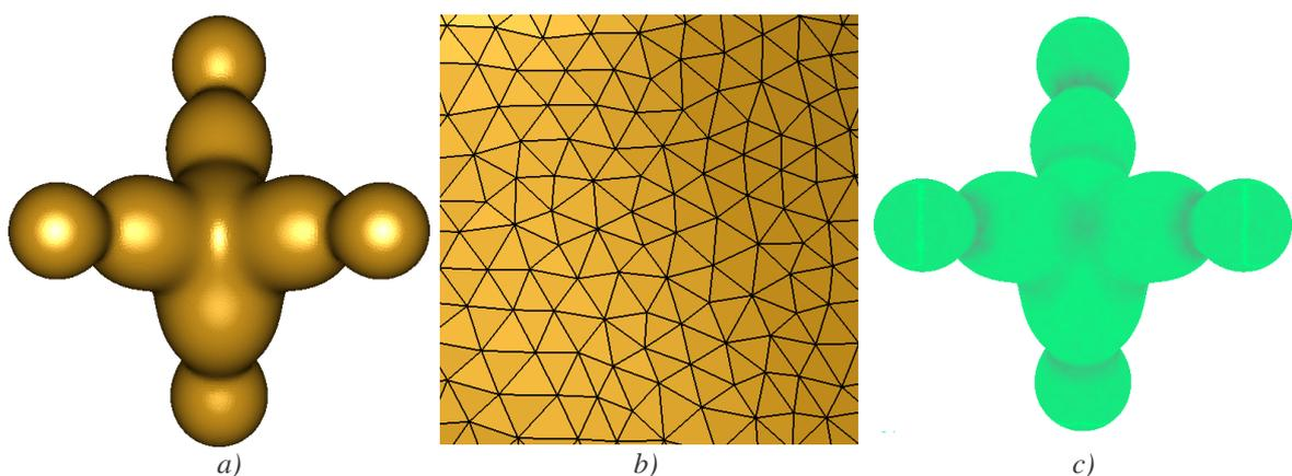
Fig. 5.2: a) An example of the reconstruction of a uniformly scanned object, b) the detail of the reconstructed surface with a triangle mesh, c) the  $\varepsilon$ -sampling of the surface, all places passed the LFS sampling criterion.
