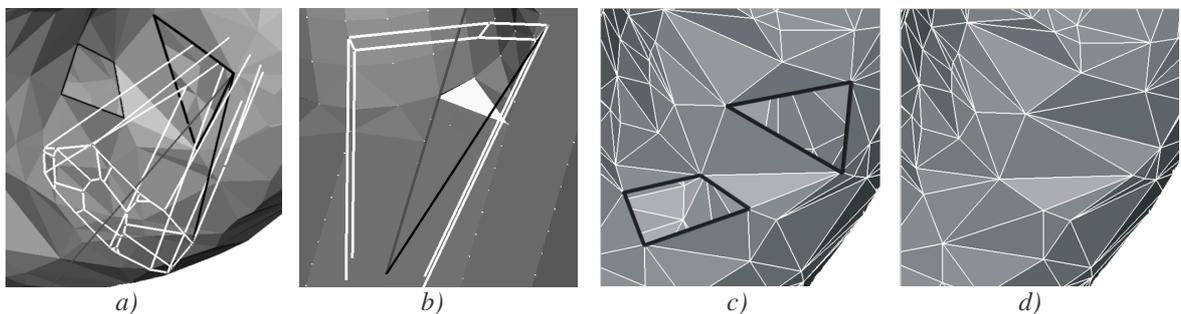
Fig. 8.3: a), b) Two examples of Voronoi cells with original estimated normal vectors (black lines) and average normal vectors (gray line), c) a part of a surface reconstructed using original normal estimation with holes in the surface, d) the same part of a surface reconstructed using average poles, the holes disappear.
