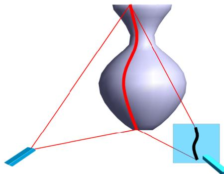
*Fig. 1.1: Principle of  $E^3$  scanning by laser scanner.*
