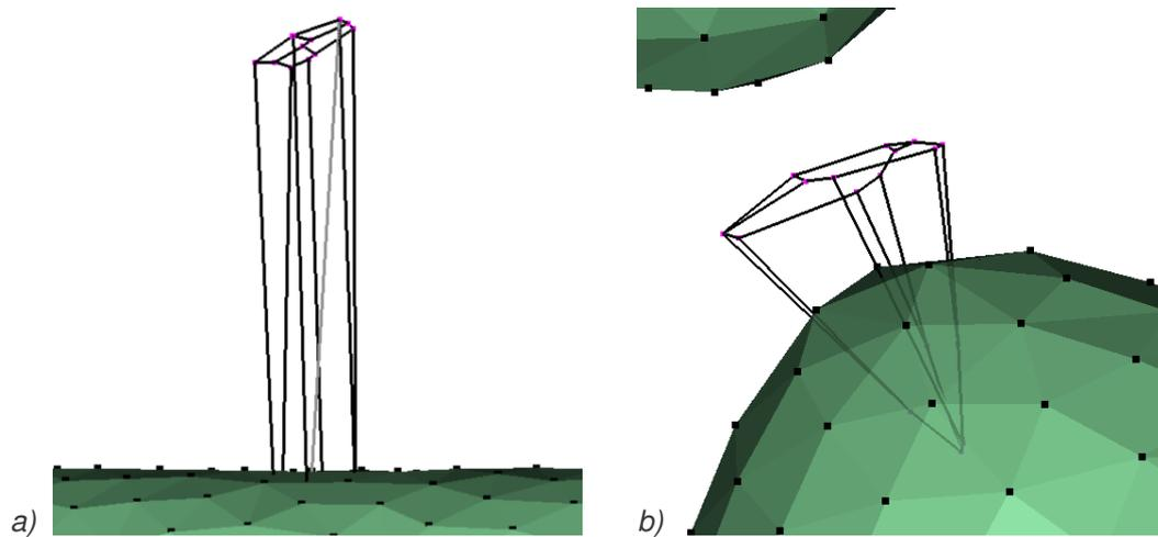
Fig. 4.5: Examples of the Voronoi cells on the reconstructed surface, a) the Voronoi cell of some point in a flat part of some surface (the gray line presents the normal vector estimated using the positive pole), b) the Voronoi cell of some point in the place where two surfaces are close (the normal vector is not visible, it directs down to the sharp edge of the Voronoi cell).
