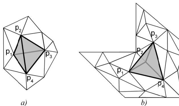
Fig. 8.5: Two examples where overlapping triangles may appear, a) a flat part of the surface, b) a part with a sharp edge. One pair of triangles is  $p_1p_2p_3$  and  $p_1p_3p_4$ , the second pair is  $p_1p_2p_4$  and  $p_2p_3p_4$ .
