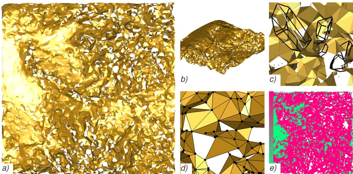
Fig. 5.6: a) An example of the surface with noise, b) another view of the surface, c) the Voronoi cells of some points in the surface, d) the detail of the reconstructed triangle mesh, e) the  $\varepsilon$ -sampling of the surface.
