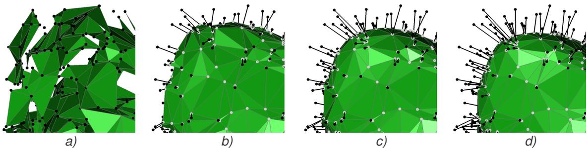
Fig. 7.9: The reconstruction of noisy data, white points are moved denoised points, black points present the original positions of points, a) the reconstruction without denoising, b) after one iteration, c) after two iterations, d) after three iterations.
