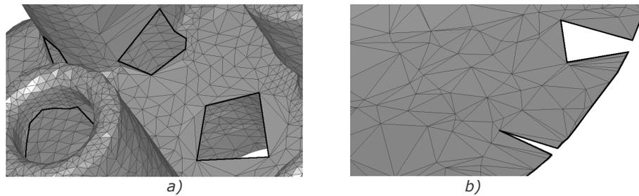
Fig. 9.18: Typical holes, a) small holes which have to be triangulated, b) boundary holes, only a few of triangles have to be added to correct the shape.
