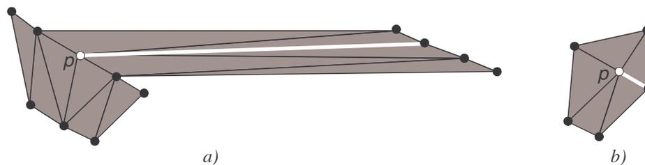
Fig. 9.9: a) The referential edge is taken as the median of all edge lengths (the white edge), b) the referential edge is the shortest edge.
