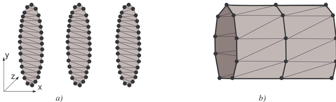
Fig. 5.3: a) An example of the object sampled in one direction more precisely than in others, b) uniformly sampled object (in both directions almost the same resolution).
