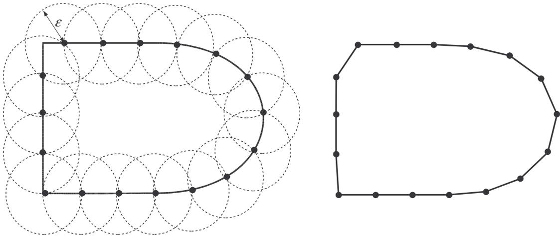
Fig. 1.3: The object and its sampling using the sampling path. The circles with the radius  $\varepsilon$  show the sampling path, the reconstruction is shown in the right part of the figure where a badly reconstructed corner appears.
