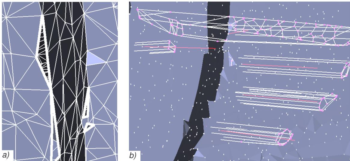
Fig. 5.7: The reconstruction of a sharp edge, a) a detail, b) the Voronoi cells near the sharp edge have required properties but the cells at the points on the edge have bad shape (not thin in one direction).
