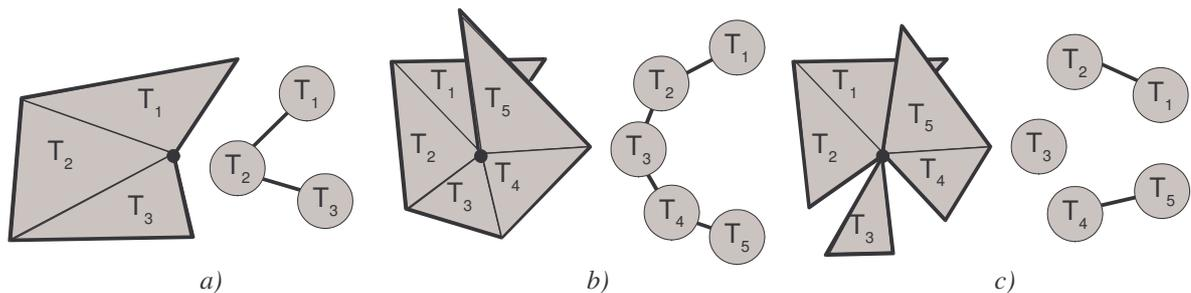
Fig. 9.5: Some fan configurations formed only by subfans, a) one subfan without overlapping triangles in a projection, b) one subfan with overlapping triangles in a projection, c) more subfans.
