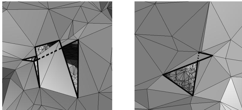
*Fig. 9.7: The overlapping triangles in the surface reconstructed using COCONE algorithm.*
