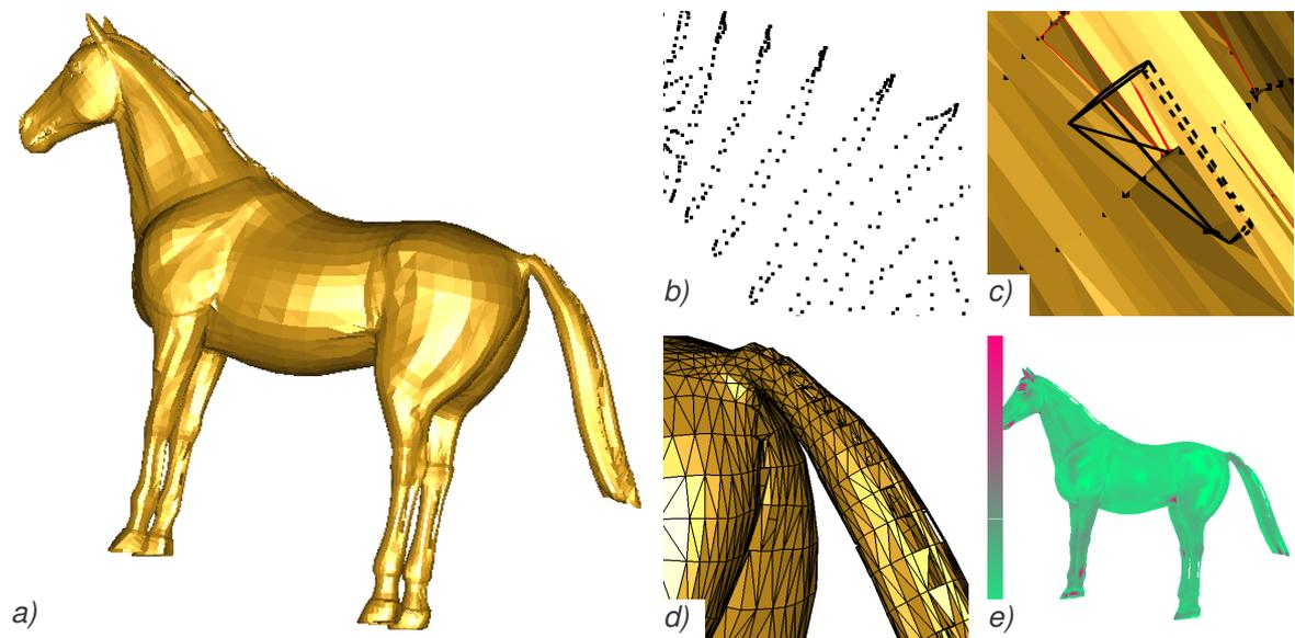
Fig. 5.4: a) An example of the uniformly scanned object, which is scanned in some regions more densely in one direction, b) the distribution of points in the neck part, c) the Voronoi cell of some point in the neck part (the estimated normal is not orthogonal to the surface), d) the tail part of the object with the triangle mesh, e) the  $\epsilon$ -sampling, darker places have bad LFS.
