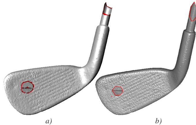
Fig. 9.16: a) The club dataset reconstructed by COCONE, the reconstruction is correct and boundaries triangles were removed, b) the reconstruction by our approach, boundary triangles successfully removed, too.
