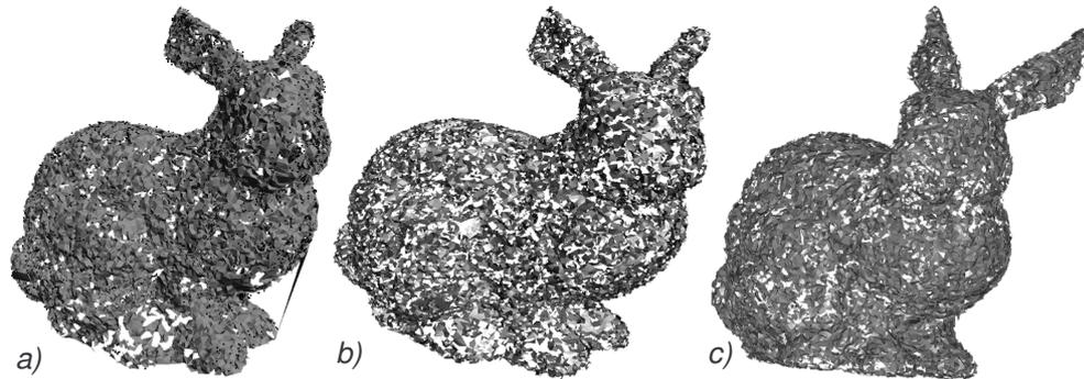
Fig. 7.3: The unsuccessful surface reconstruction of a noisy dataset, a) by the INRIA surface reconstructor, b) by the COCONE, c) by our CRUST implementation without points denoising.
