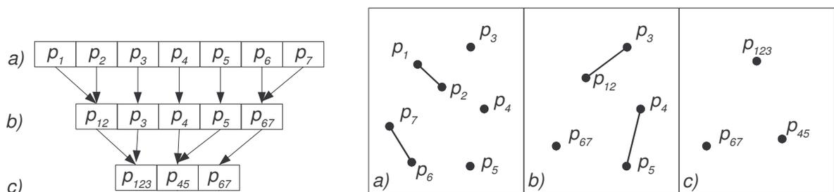
Fig. 12.1: The points decimation procedure with three iterations and the graph related to each iteration.
