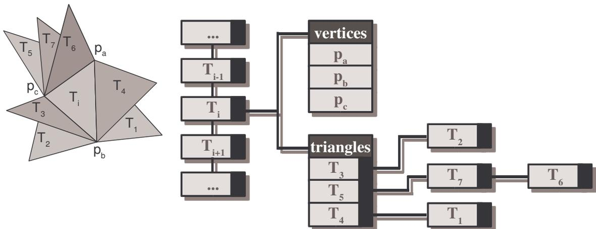
Fig. 8.7: An example of the structure which contains for each triangle the list of all possible triangle neighbours on its edges.
