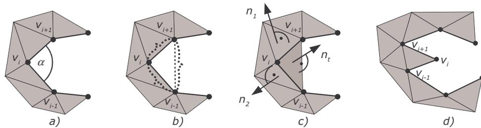
Fig. 9.20: The ear  $v_{i-1} v_i v_{i+1}$  evaluation, a) the smallest angle,  $\alpha_i$  is the angle between the vector  $v_{i-1} - v_i$  and the vector  $v_{i+1} - v_i$ , b) the smallest length of the edges, c) the smallest angle between neighbours,  $n_1$  is the normal vector of the triangle with the edge  $v_{i+1} v_i$ ,  $n_2$  is the normal vector of the triangle with the edge  $v_{i-1} v_i$ ,  $n_t$  is the normal vector of the ear, d) an invalid ear.
