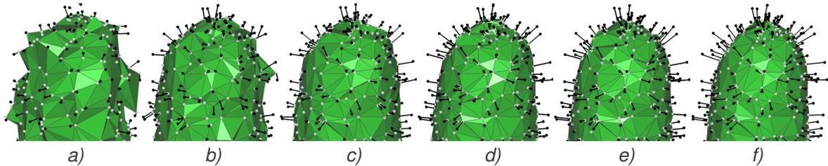
Fig. 7.10: The reconstruction of noisy data, white points are denoised points, black points show the original position, a)  $k = 5$ , b)  $k = 10$ , c)  $k = 15$ , d)  $k = 20$ , e)  $k = 25$ , f)  $k = 30$ .
