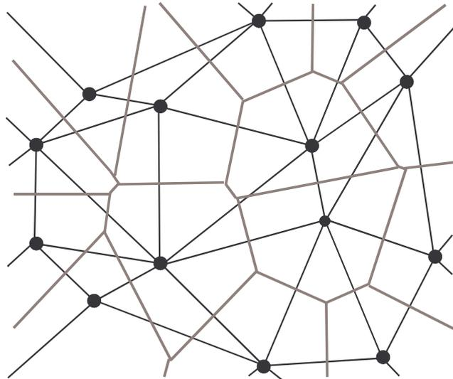
Fig. 2.6: A planar example of Voronoi diagram in gray and Delaunay triangulation in black.
