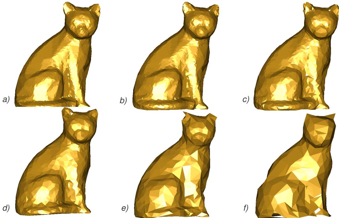
Fig. 7.13: The test of the points decimation before the reconstruction, a) the reconstruction of the original point cloud with 10000 points, b) 5000 points, c) 2500 points, d) 1250 points, e) 600 points, f) 300 points.
