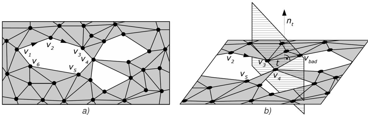
Fig. 9.17: Holes tracing, a) the vertices  $v_1v_2v_3v_4v_5v_6$  represent the hole, the vertex  $v_4$  is problematic, b) the plane created using the edge  $v_3v_4$  and a triangle  $t$  (with normal  $n_t$ ) coincident to the edge, the vertex  $v_{bad}$  is the vertex with the smallest angle to the edge  $v_3v_4$ .
