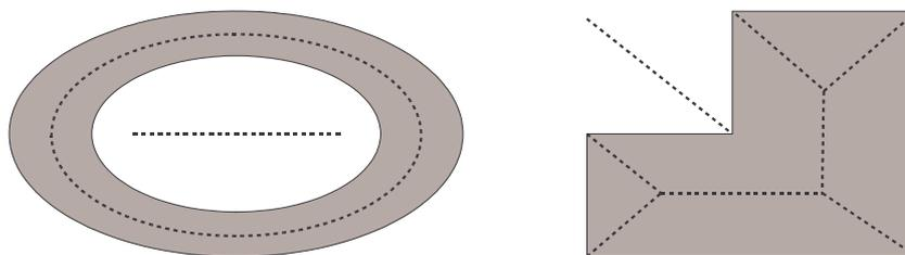
Fig. 2.3: The medial axes (dashed line) of two objects.
