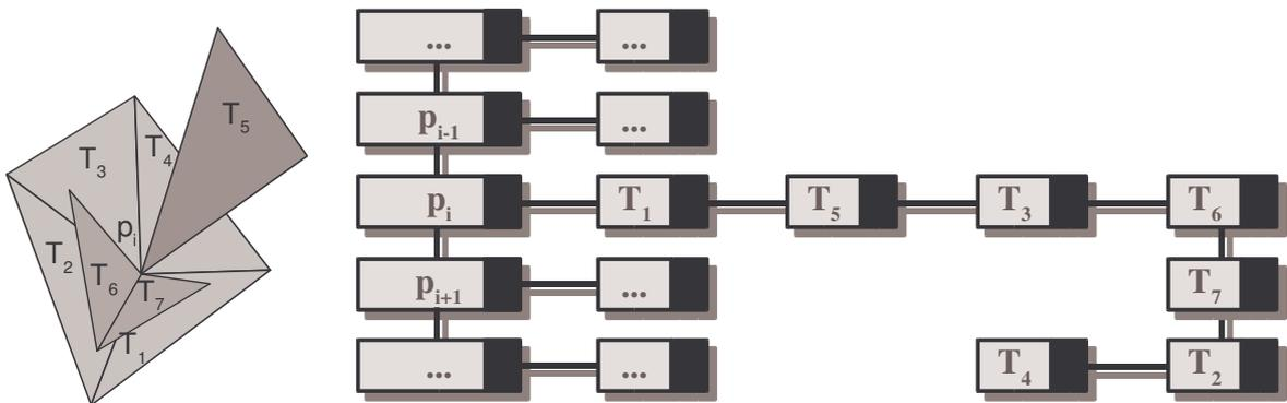
Fig. 8.6: An example of the data structure where each point  $p_i$  has a list of its incident triangles  $T_i$ .
