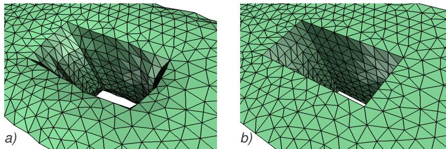
Fig. 7.11: The use of denoising in the reconstruction of sharp edges, a) the reconstruction after denoising without points translation, b) with points translations.
