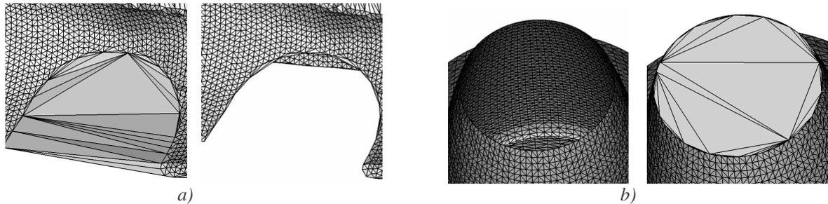
Fig. 9.12: a) An example of the boundary filtering when the boundary triangles are parallel with the surface triangles, b) when the boundary triangles are perpendicular to the surface triangles.
