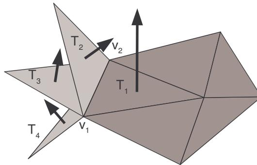
Fig. 8.8: The dark gray triangles have been already extracted, the light gray triangles  $T_2$ ,  $T_3$ ,  $T_4$  are incident on one edge to the triangle  $T_1$  and one of them has to be chosen.
