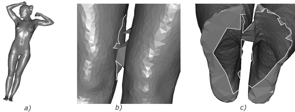
Fig. 9.23: The datafile with problematic connected places, a) the whole surface, b) the legs with big point undersampling, c) the feet with the same problem.
