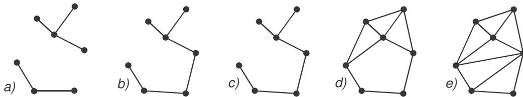
Fig. 2.4: The comparison of the subgraphs of Delaunay triangulation, a) NNG, b) EMST, c) RNG, d) GBG, e) DT.
