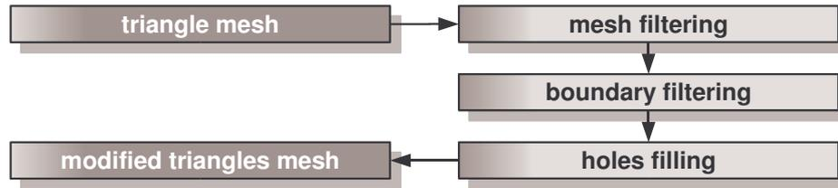
*Fig. 6.4: The triangle mesh filtering steps.*
