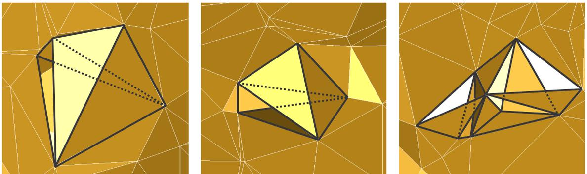
*Fig. 9.1: Some parts of the reconstructed surface with errors after manifold extraction.*
