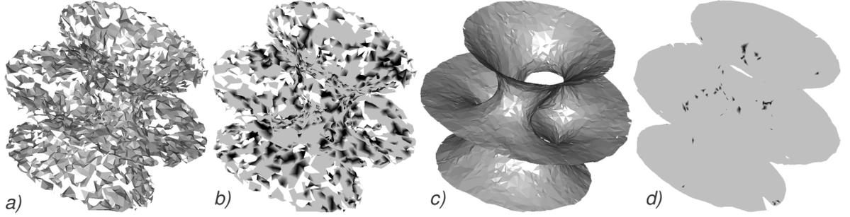
Fig. 7.6: The surface reconstruction of a noisy dataset, a) badly reconstructed surface without denoising, b) the LFS of the surface from a), c) the reconstruction after Laplacian denoising, d) the LFS of the surface from c).
