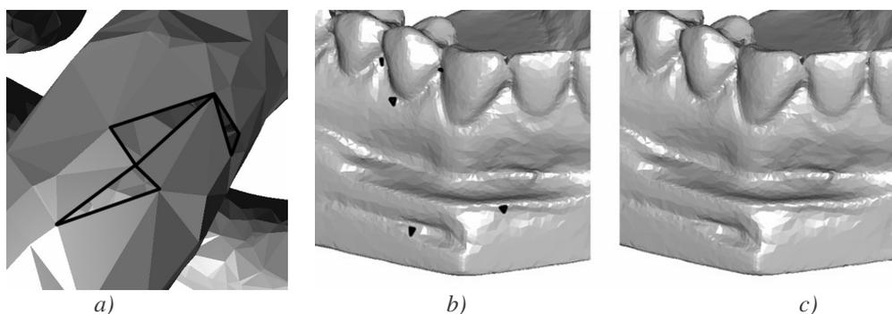
Fig. 8.13: a) The detail to the surface reconstructed by Dey's COCONE, triangle holes in the surface are black, b) shows the reconstruction by our algorithm without the help of prefiltering (missing triangles are black) and c) with the help of prefiltering.
