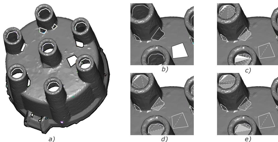
Fig. 9.21: The result of the holes filling, a) the whole mesh with holes highlighted, b) a zoom to one part with holes, c) the smallest angle filling, d) the smallest edge length filling, e) the smallest neighbours angle.
