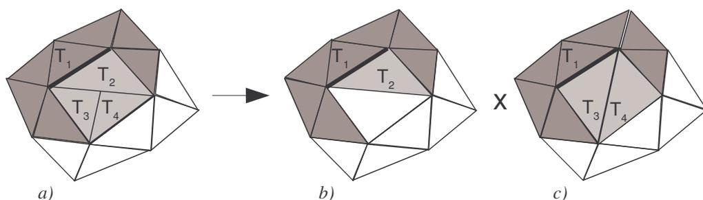
Fig. 8.11: Two configurations in the manifold extraction of the tetrahedron with three marked surface triangles, a) the initial status, on one edge of the triangle  $T_1$  there are two connected triangles belonging to one tetrahedron, b) the wrong choice, c) the correct choice.
