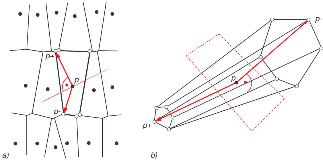
Fig. 4.1: The point  $p$ , the Voronoi cell and Voronoi vertices around it in  $E^2$  and  $E^3$ . The vertex  $p+$  is the positive pole, because it is the farthest vertex from the point  $p$ , the vertex  $p-$  is the negative pole, it is the farthest vertex on the “other side”.
