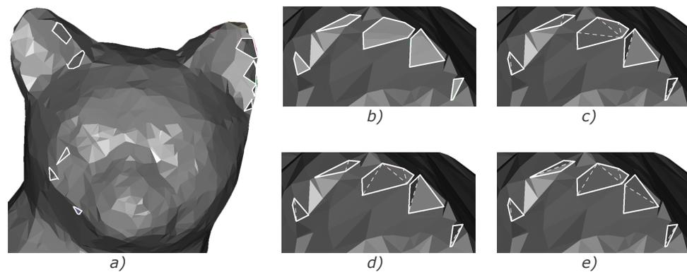
Fig. 9.22: The result of the holes filling, a) the head of the cat with highlighted holes, b) a zoom to one ear with holes, c) the smallest angle filling, d) the smallest edge length filling, e) the smallest neighbours angle.
