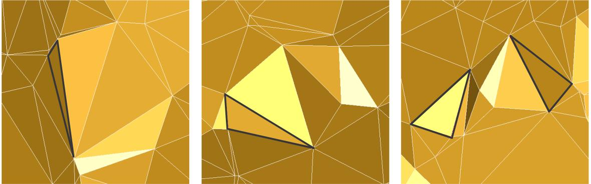
*Fig. 9.6: The same parts of the surface as in Fig. 9.1 after applying prefiltering. The black triangles present the triangle holes formed after postfiltering which were filled with triangles.*
