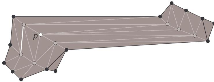
Fig. 9.10: Current selection of referential edge (white edge) of a point  $p$ , grey edges are the edges from which referential edge as a median was selected, points in grey are the neighbours of point  $p$ .
