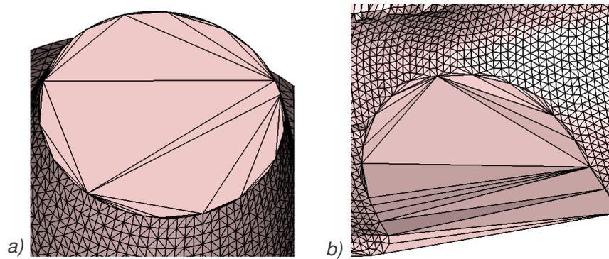
Fig. 9.8: Two examples of badly triangulated boundary, a) the boundary triangles perpendicular to the surface triangles, b) the boundary triangles parallel to the surface triangles.
