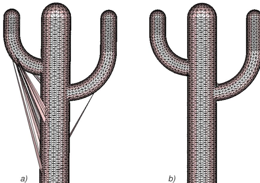
Fig. 5.1: a) An example of the reconstruction without using the numerically stable Delaunay tetrahedrization, b) the reconstruction with numerically stable Delaunay tetrahedrization.
