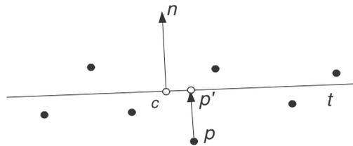
Fig. 7.7: The process of denoising,  $k$  nearest neighbours for the point  $p$  are used for the centroid  $c$ , tangent plane  $t$  and normal vector  $n$  computation, the point  $p$  is transformed to  $p'$  lying in the tangent plane in the direction of  $n$ .
