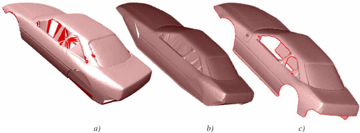
Fig. 9.13: a) The model reconstructed by the COCONE, detected boundaries are the highlighted parts, b) the same model reconstructed using CRUST without any boundary improvement, c) after applying the boundary filter; highlighted parts are traced boundary edges.
