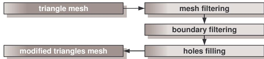
*Fig. 6.4: The triangle mesh filtering steps.*
