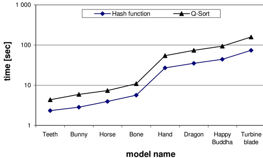
Figure 6-5: Achieved time comparison for two mentioned approaches. Presented Q-Sort time was achieved running on 8 processors, while bucketing function time is valid for sequential run on one processor.
