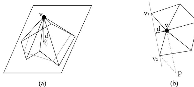
Figure 5-3: Distance  $d$  for vertex importance evaluation, (a) - simple vertex case, (b) - boundary vertex case.
