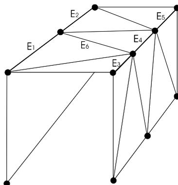
Figure 7-11: An example of sharp edge (E1-E5) and flat edge (E6).
