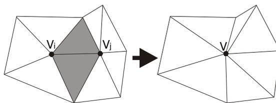
Figure 4-7: Edge ( $v_i, v_j$ ) is contracted. The dark triangles become degenerate and are removed.
