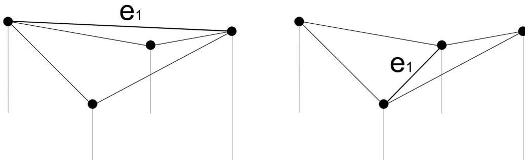
Figure 5-1: Two possibilities of placing edge  $e_1$  to triangulate the area among four vertices.
