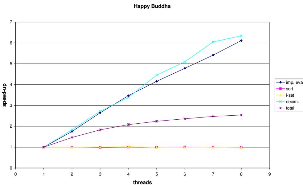
Figure 6-2: The speed-up of partial phases of the simplification algorithm.
