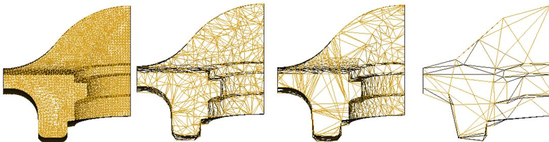
Figure 7-13: Example of reduced model. The original mesh (left), 90% reduction with and without vertex memory (two in the middle) and drastical 99% reduction (right).
