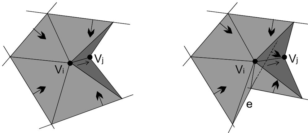
Figure 5-5: The new vertex ( $v_j$ ) must lie on the same half-plane of all oriented edges to prevent fold-over.
