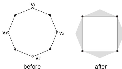
Figure 6-10: Shrinkage caused by the removal of vertices  $v_1$ ,  $v_2$ ,  $v_3$  and  $v_4$ .
