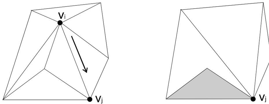
Figure 2-10: Edge collapse leading to nonmanifold mesh.
