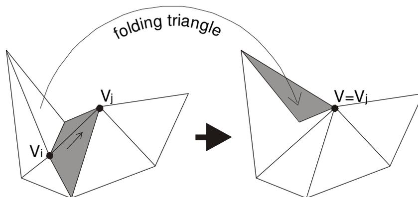
Figure 2-9: An edge contraction, which causes the mesh to fold over on itself.
