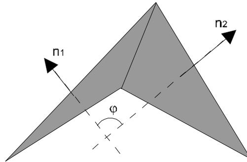
Figure 5-4: Spatial angle  $\varphi$  of two triangles is given by the angle between their normals.
