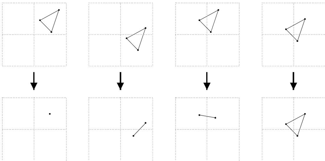
Figure 3-2: Several examples of vertex mapping while clustering one triangle.
