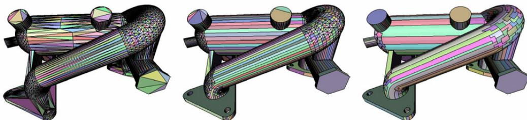
Figure 2-11: Face cluster partitions produced by iterative pair-wise merging (taken from [12]); original 11,036 clusters (left), 6000 clusters (middle), 1000 clusters (right).
