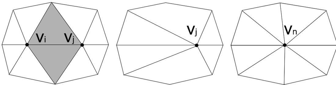
Figure 2-8: Edge collapse operator; original mesh (left), half-edge collapse (middle), full-edge collapse (right).
