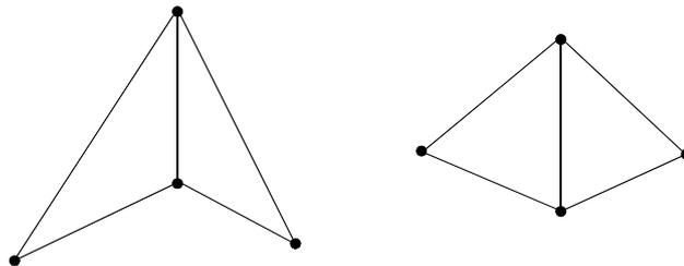
Figure 7-8: The arrow-shaped quad (left), the non-problematic case (right).
