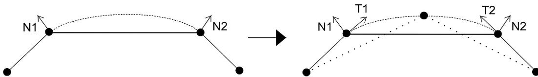
Figure 7-7: The new vertex should lie somewhere on the dashed line (in 2D).
