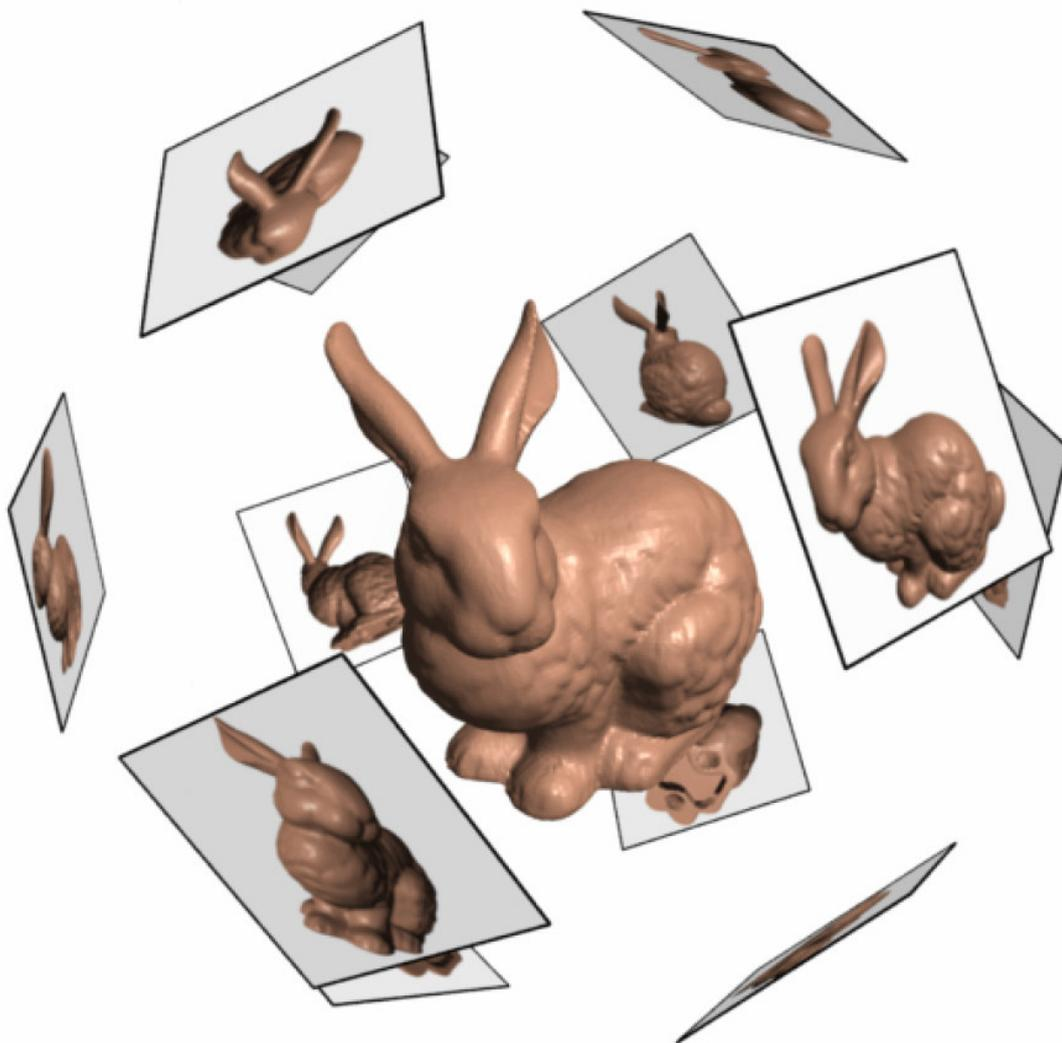
Figure 4-8: Twelve uniformly distributed views of a model. The viewpoints correspond to the vertices of a regular icosahedron (taken from [32]).
