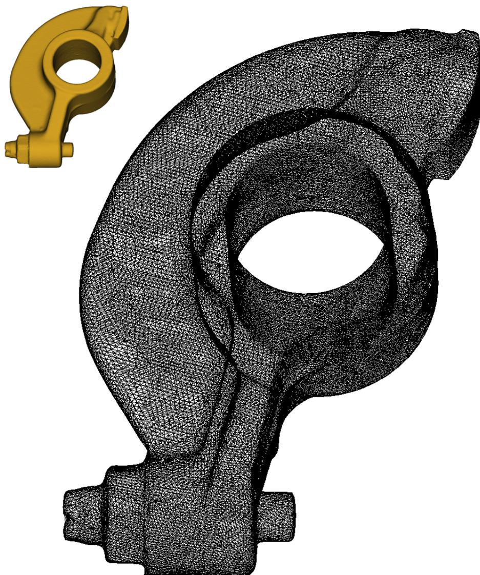
Figure 2-1: The example of polygonal surface model (courtesy Cyberware). This original model contains 40117 vertices and 80354 triangles.
