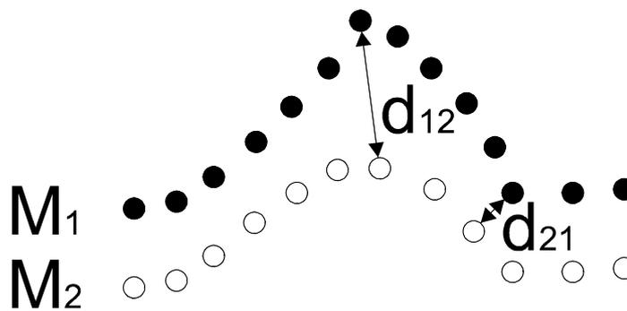
Figure 3-1: The Hausdorff distance between two surfaces  $M_1$  and  $M_2$ .
