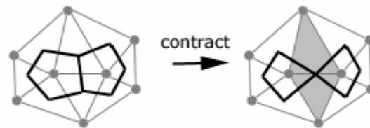
Figure 4-4: Edge contraction in the dual graph. The two faces of the surface corresponding to the endpoints of the dual edge are merged to form a single face cluster.
