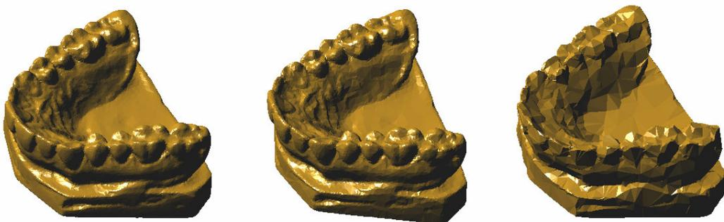
Figure 6-7: A teeth model (courtesy Cyberware) at different resolutions; the original model with 58,328 triangles on the left, reduced to approx. 29,000 triangles in the middle and 6,000 triangles approximation on the right.
