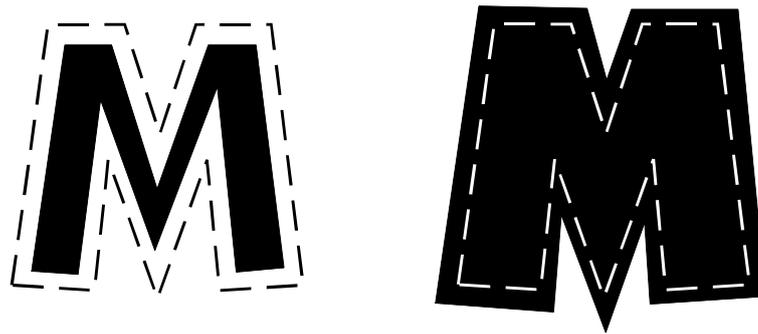
Figure 2-13: Erosion and dilatation in 2D.
