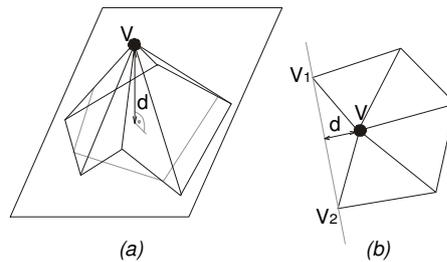
Figure 4-6: The distance between a vertex and the average plane (a) and between a vertex and the bisector (b).
