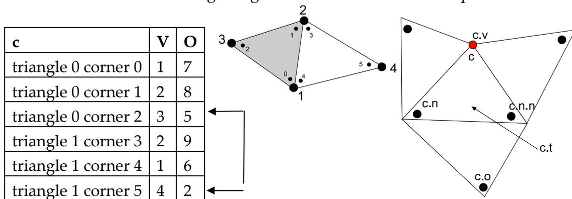
Figure 2-14: Vertices and corners in corner-table scheme.
