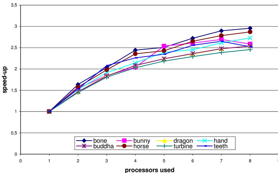
Figure 6-1: The speed-up of total computation (total time), parallel and sequential parts together; the acceleration is computed for several models of different amount of triangles.
