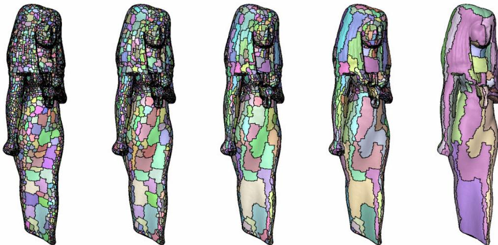
Figure 4-5: Face clusters computed for Isis statue, composed of 375,736 triangles. Cluster shape adapts to surface shape. From left 10,000 clusters, 5000 clusters, 2500 clusters, 1000 clusters and 100 clusters.
