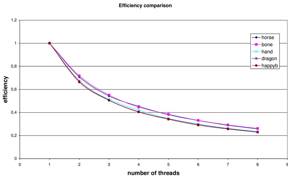
Figure 6-3: The efficiency of total computation; the efficiency is computed for several models of different amount of triangles.
