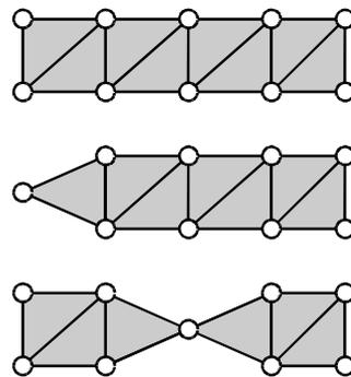
Figure 2-4: Two approximations of the same surface, both constructed by contracting a single edge (top – original, middle – manifold, bottom – non-manifold).
