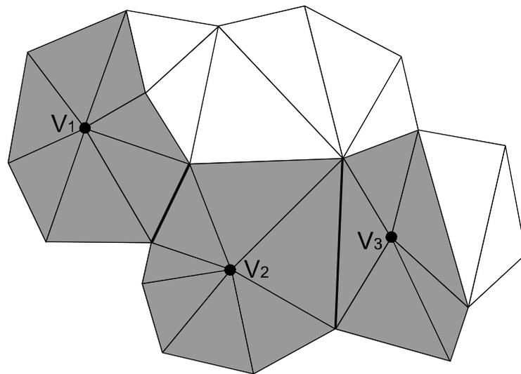
Figure 5-6: Vertices  $v_1$ ,  $v_2$ ,  $v_3$  are independent to each other; vertices  $v_1$  and  $v_3$  are super independent.
