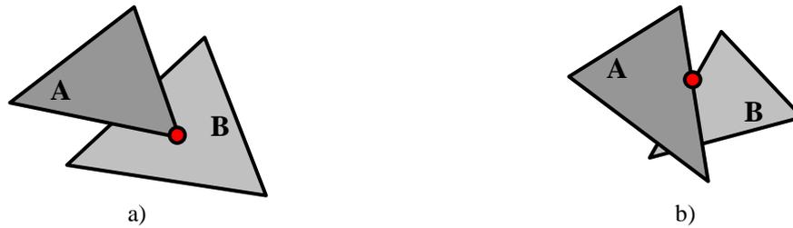
**Figure 7.3:** Two possible types of triangle vs. triangle collision – a) vertex of one triangle collides with the other triangle, b) two triangles collide by edges.
