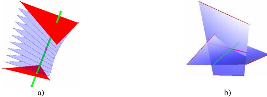
**Figure 7.1:** a) a collision between a triangle under linear motion and a point moving along linear trajectory, b) a collision between two edges, where each vertex of the edge moves independently along a linear trajectory.
