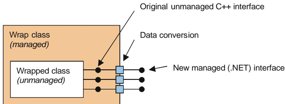
Figure 4.2 – Wrap-class contains wrapped class and suits its interface into .NET manner
