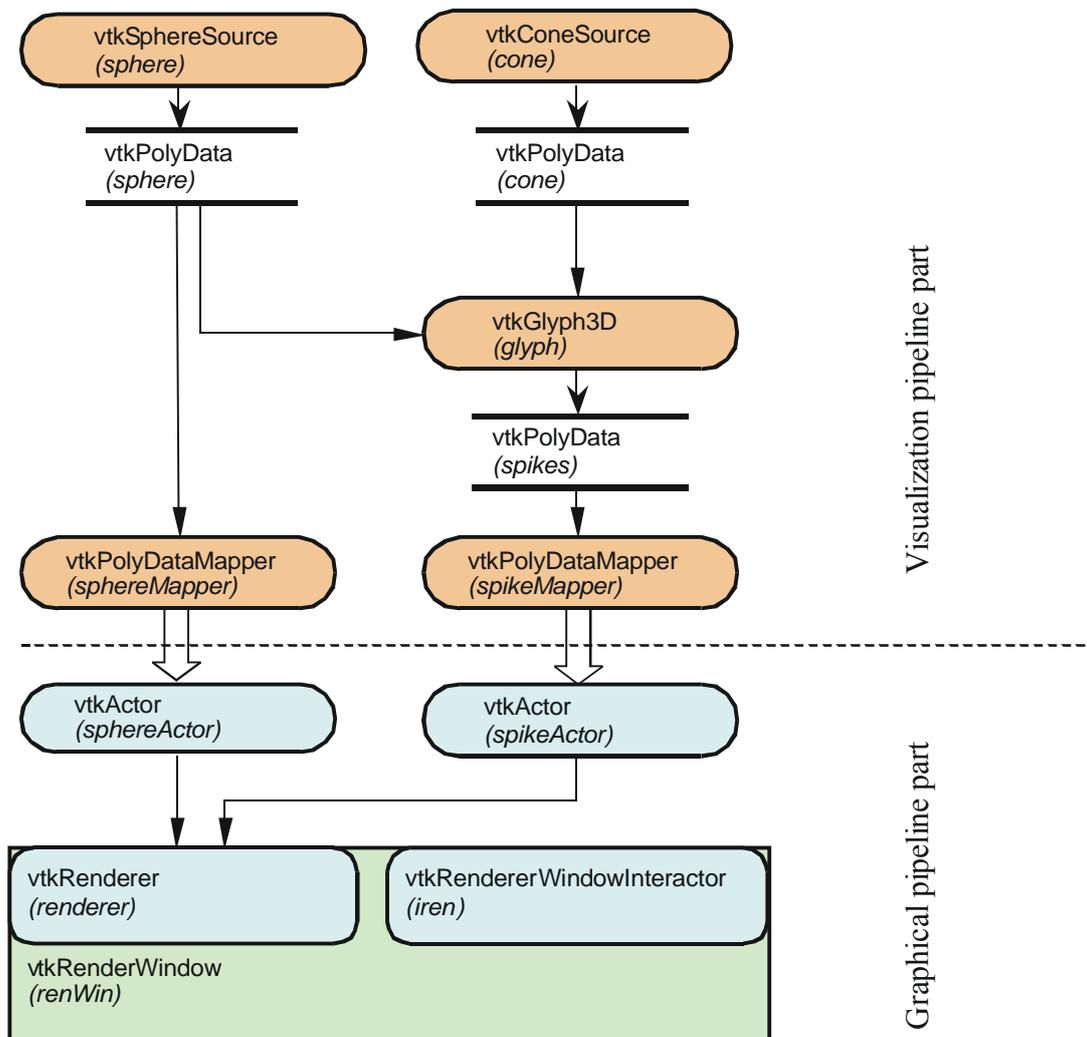
Figure 2.7 - The mace example as with visualization pipeline and graphical part
