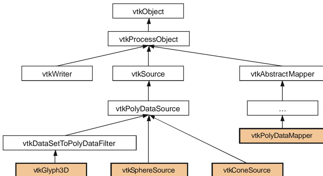
Figure 2.8 – Used process objects as inheritance graph. Instanced object are highlighted
