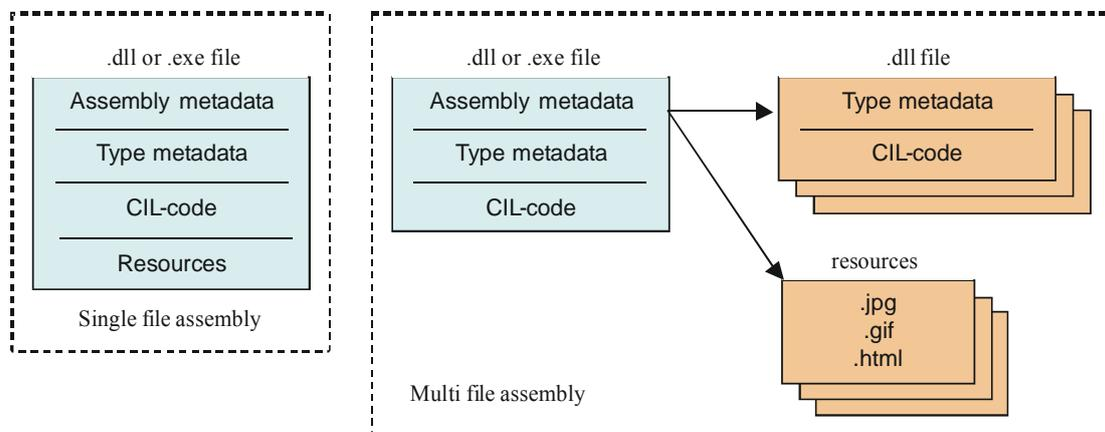
Figure 3.3 – Single- and multi- file assembly structure
