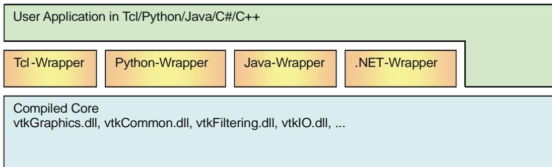
Figure 2.9 - Core, wrappers, and user application. Note the direct access possibility
