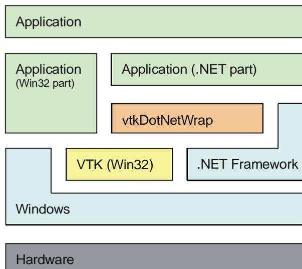
Figure 4.1 – Placement of interfacing layer in resulting application
