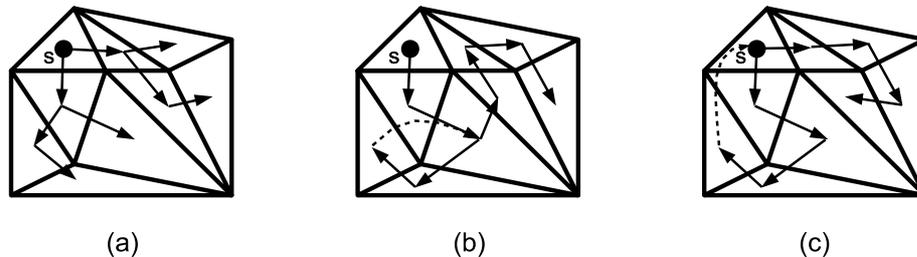
Figure 3.7: Three approaches for the construction of spanning tree. Standard breadth-first search BFS (a), depth-first search BFS (b) and a hybrid search (c).  $S$  is the root node of the spanning. A dashed line represents returns in the graph search algorithm. (From [39])
