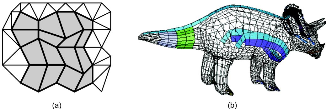
Figure 3.5: An example of a rectangular patch (a) and a typical polyhedral mesh with patches (b). (From [16])
