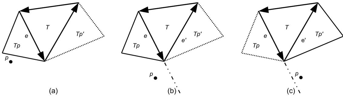
Figure 3.8: If the closest point to point  $p$  is an inner point of the edge  $e$  of the triangle  $T$ , then  $T_p$  is the predecessor of  $T$  (a). If the edge  $e$  is exposed to  $p$ , then  $T_p$  is the predecessor of  $T$  (b) else  $T'_p$  is predecessor of  $t$  (c). (From [30])
