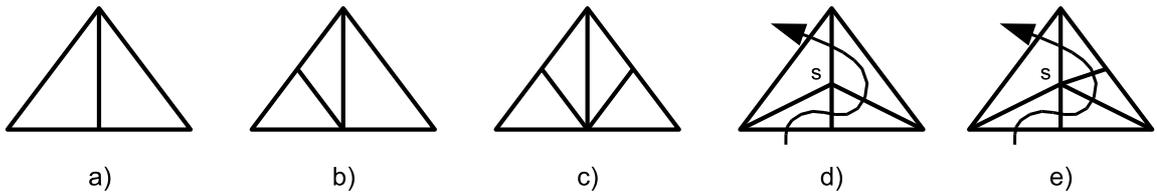
Figure 3.17: For non-uniform subdivision, three templates splitting one (a) two (b) and three (c) edges exist. In two situations it is not possible to produce a triangle sequence, thus the subdivision template has to be modified by inserting a Steiner point  $s$  (d,e). (From [36])
