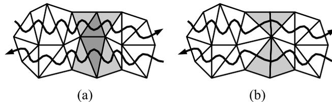
Figure 3.13: A triangulation and its stripification (a). In the case of a good stripification, the strips are preserved during the simplification process (b). (From [5])
