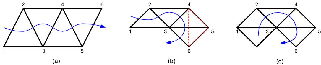
Figure 2.1: An example of a sequential triangle strip (a), a generalized triangle strip (b) and a triangle fan (c).
