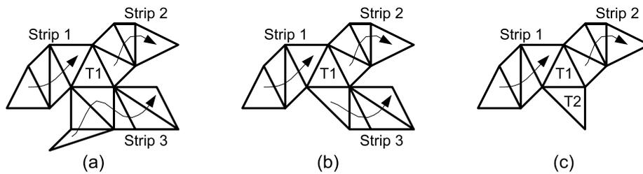
Figure 3.3: Concatenation rules in da Silva's algorithm: If a triangle of degree 0 is adjacent to two strip extremities, the strips are concatenated (a), if it is adjacent to three strip extremities, the concatenation that does not produce a swap is chosen (b). If a triangle of degree 1 is adjacent to two strip extremities and to other triangle, the concatenation depends on the degree of the neighboring triangle (c). (From [29])
