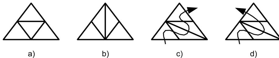
Figure 3.16: Isotropic subdivision template (a). Anisotropic subdivision template (b). Triangle sequences in anisotropic template (c,d). (From [36])
