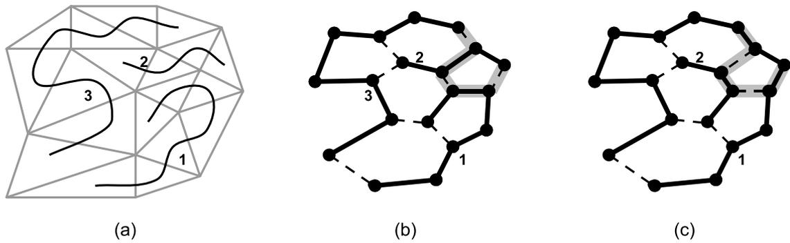
Figure 3.10: A triangle mesh with three strips (a). The tunnel (gray) is an alternating sequence of strip (solid) and nonstrip (dashed) edges (b). Complementing the status of edges in the tunnel, the number of strips is reduced by one (c). (From [32])
