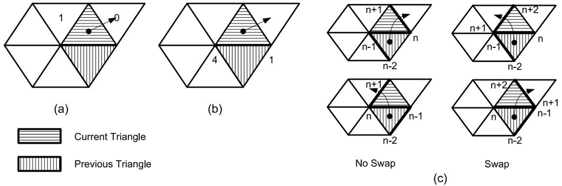
Figure 3.2: Three types of heuristic functions in Kornmann's algorithm. A mesh connectivity criterion (a), a vertex connectivity criterion (b) and vertices minimizing criterion (c). (From [24])
