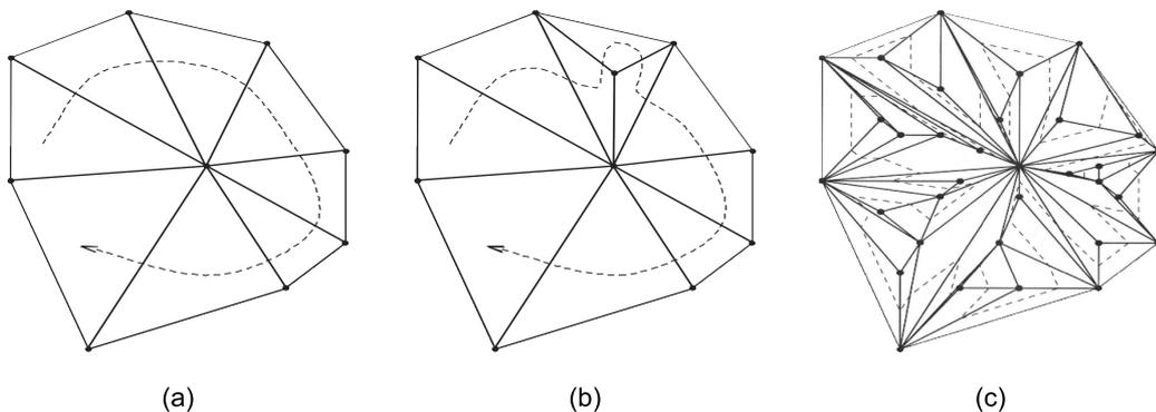
Figure 3.14: The initial triangulation contains the convex hull and one inner point (a). While inserting the remaining vertices, the strip can be preserved (b). The final triangulation contains only one strip (c). (From [3])
