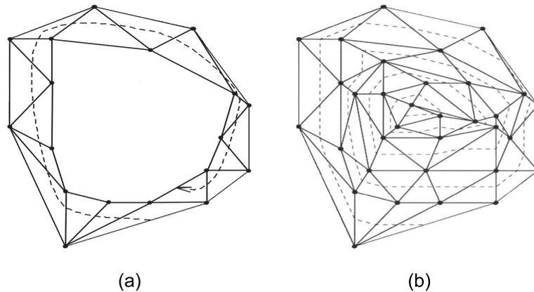
Figure 3.15: The annulus bounded by the first and the second convex hull is triangulated and a strip connecting all triangles is created (a). Following the same construction scheme, the whole triangulation can be created (b). (From [3])
