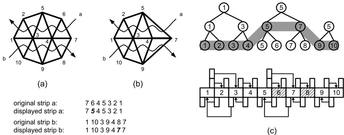
Figure 3.19: An original mesh covered by two strips (a), A decimated mesh (b) and corresponding merge tree and skip list (c). The dark area in the merge tree shows the active LOD for the mesh. (From [13])
