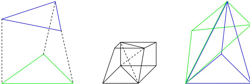
**Figure 19: Moving triangle as a 4D prism (green is the triangle in time  $t$ , blue is the triangle in time  $t+1$ ), two possible diagonals on a common side, two tetrahedra used for consistent subdivision.**
