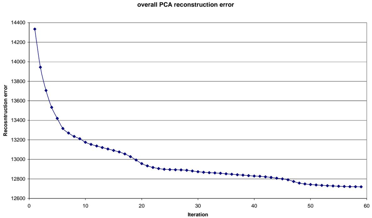
Figure 23: convergence of the CPCA error during the iterative clustering improvement procedure.
