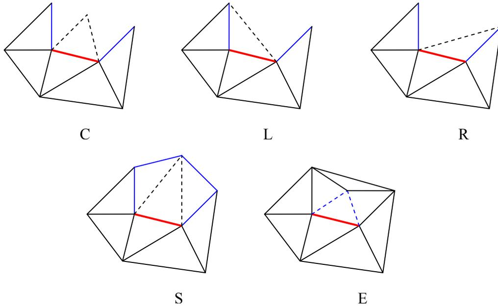
**Figure 8: EdgeBreaker cases. Red edge represents the gate, blue edges belong to the current border.**
