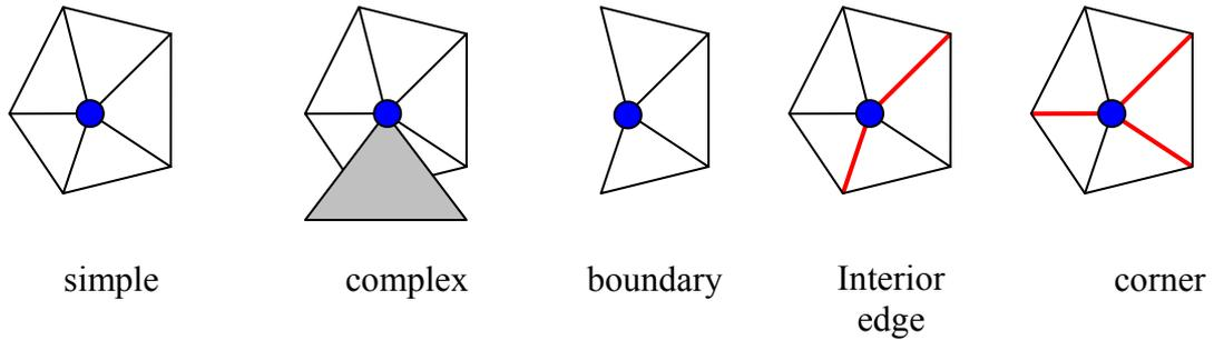
**Figure 9: local geometry and topology characteristic for decimation.**
