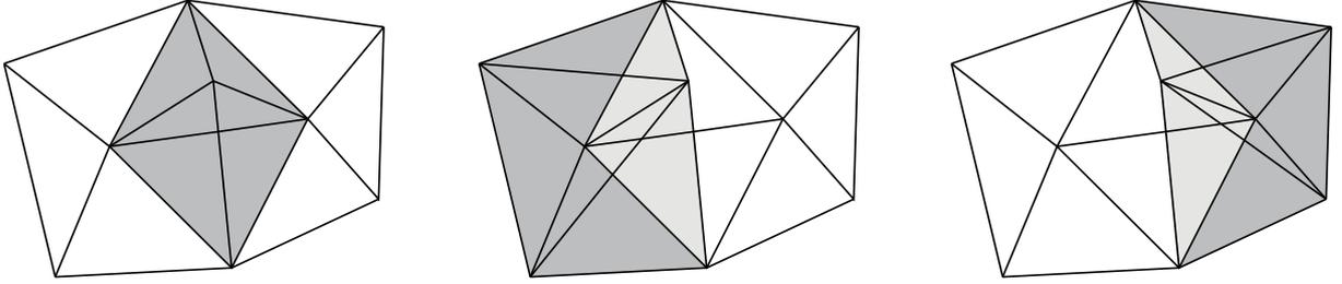
**Figure 16: Tetrahedra created in the neighborhood of a contracted edge, from left to right two tetrahedra incident with the removed triangles, tetrahedra incident with vertex  $v_1$  and tetrahedra incident with vertex  $v_2$ .**
